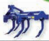
3 TYNE - SUB SOILER
