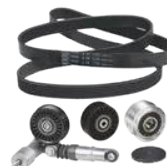
Multi-V belt kits with freewheel alternator pulley
